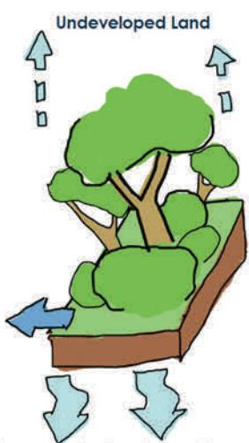
You can see much of the rainwater infiltrates into the soil or is evapotranspired back into the atmosphere.
