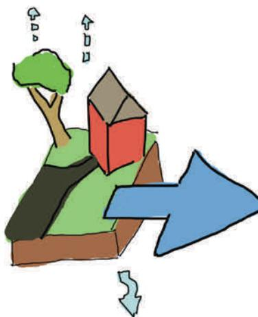
Where vegetation is replaced with streets, driveways, sidewalks, houses, and lawns, less rainwater is able to infiltrate and return to the atmosphere, and more rain turns into runoff.
