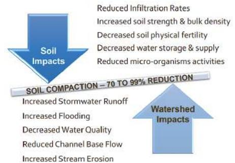
Figure 2 - Watershed Impacts from Soil Compaction
