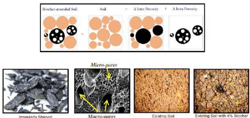
Figure 5 - Biochar and Soil Interaction Mechanism
